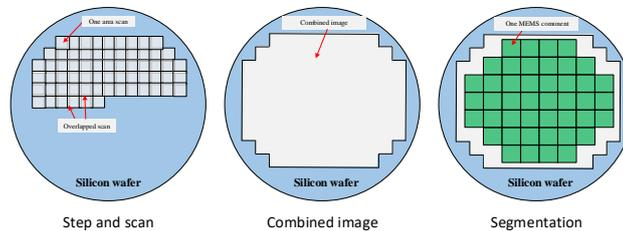
**Figure 6.** Illustration of image combination and segmentation.
