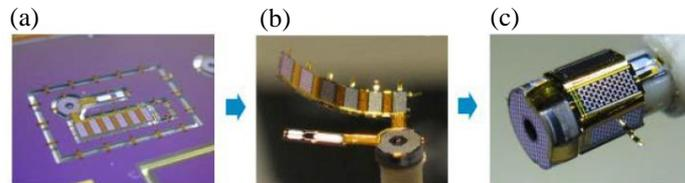
**Figure 2.** (a) F2R structures are fabricated wafer scale. (b) After fabrication the partly flexible structures are removed from the silicon wafer and assembled around a catheter tip. (c) Final 180° ultrasound microphone.
