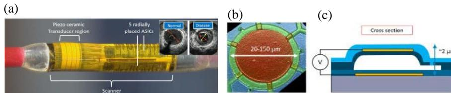
**Figure 1.** (a) IVUS scanning catheter and examples of images produced, (b) optical microphotographs of CMUT devices in top view, (c) Schematic cross-section of a CMUT.
