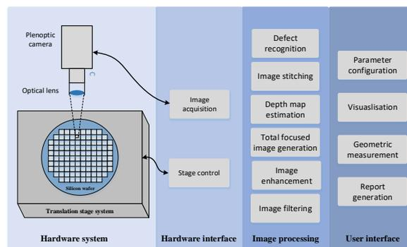
Figure 4. Schematic overview of plenoptic camera inspection sub-system.
