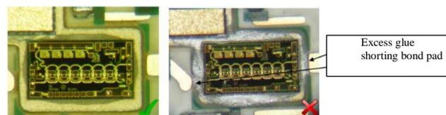
**Figure 3.** Example of failure mode as a result of incorrect adhesive dispensing.
