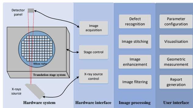
**Figure 5.** Schematic overview of X-ray inspection sub-system.
